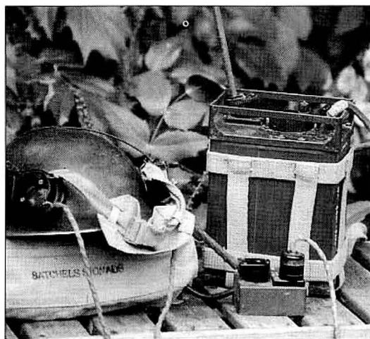
Fig. 9: The 38 set was normally carried on a webbing harness mounted on the operator's chest (see text).
